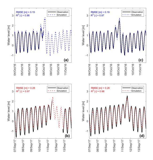
**Figure S1.** Calibration and validation of the Savannah Delft3D-FM model. Time series of simulated and observed WLs at (a, b) Port Wentworth and (c, d) Savannah River at USACE dock. Top and bottom panel show times series of Hurricane Matthew and Irma, respectively. Note that the model can simulate water level variability, and so fill the data gaps observed during Hurricane Matthew.
