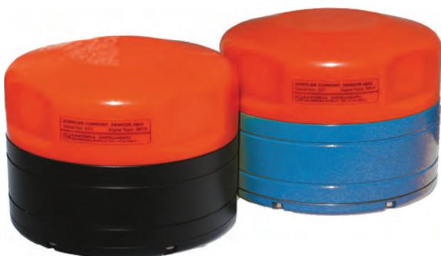
The ZPulse Doppler Current Sensor (DCS) is a single-point current sensor primarily intended to be used with the Aanderaa SeaGuard platform to form a Recording Current Meter (RCM). It is designed for commercial as well as research use. There are 8 versions; 4420/4420R, 4830/4830R has a depth rating of 300 meters, while the 4520/4520R/ 4930/4930R has a depth rating of 6000 meters. 4830/4830R/ 4939/4930R have a temperature sensor included.
