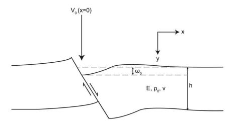
**Figure A3:** Set-up for hanging wall deflection equations. A vertical load ( $V_{\theta}$ ) is applied to the point where the hanging-wall intersects the surface (i.e., where  $x=\theta$ ) and where there is a maximum deflection ( $\omega_{\theta}$ ). The elastic thickness, Young's Modulus, density, and Poisson's ratio of the crust are represented by h, E,  $\rho_{\theta}$ , and v respectively.
