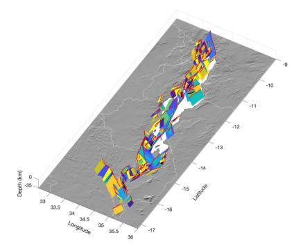
**Figure 3:** 3D geometrical model of all MSSM sources. Each coloured 2D plane represents a distinct along-strike MSSM section or fault (note colours are assigned randomly). Red and black lines are the fault traces from the Malawi Active Fault Database (MAFD) that are, and are not, included in the MSSM, respectively. Image underlain by SRTM DEM.
