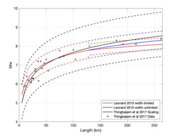
Figure 10: Length to magnitude scaling for interplate dip-slip faults Leonard, (2010). Plot includes scaling for width-limited
