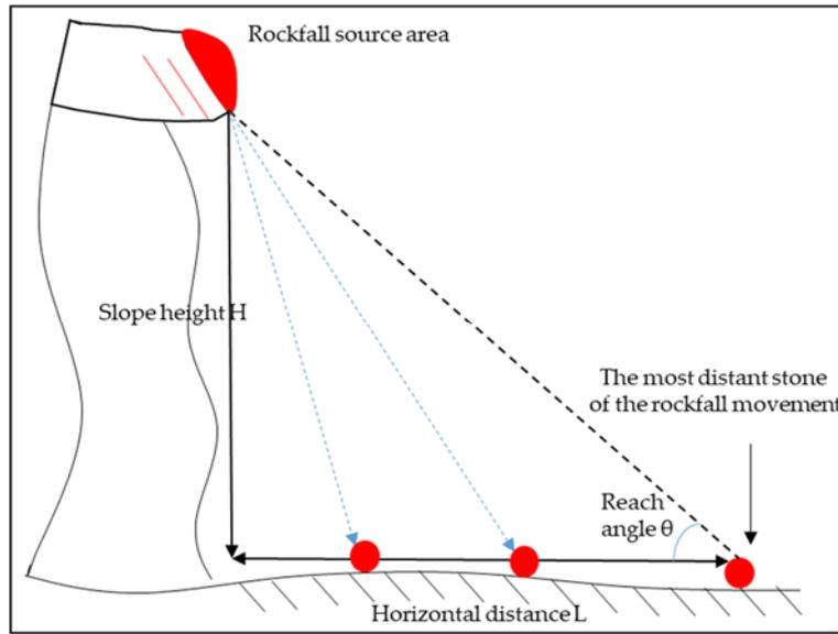
Figure 4. Reach angle diagram
