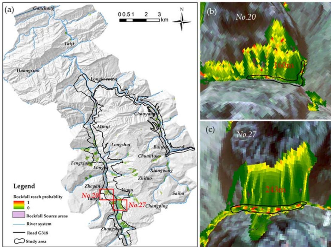
**Figure 13.** (a) Reaching probability map of rockfall along the national road G318. (b)(c) Enlarged view of partial rockfall. (Rockfall fragment distribution area is identified using black closed lines)
