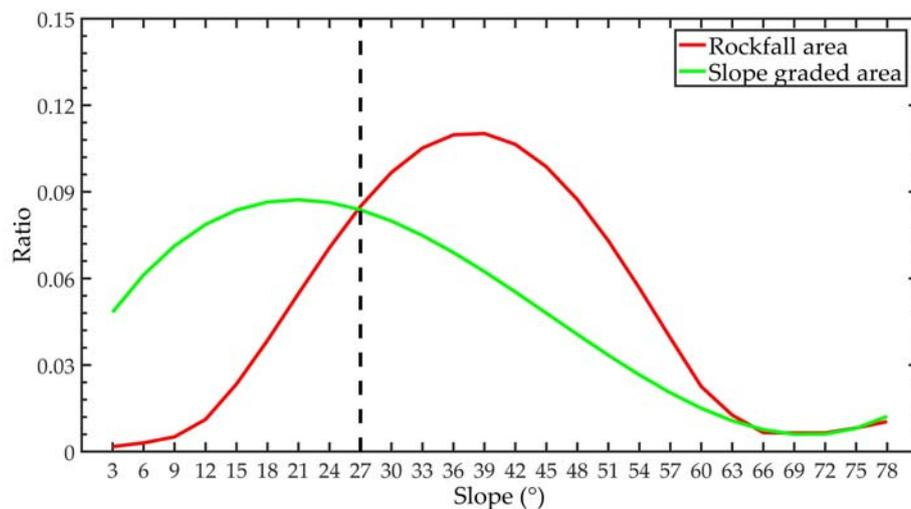
**Figure 5.** Relationship between rockfall distribution frequency and slope angle
