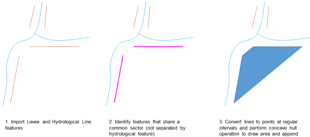
295 Figure 1: Extraction of leveed-areas from levee line information (visual representation of process outline in Supplementary Figure S3)
