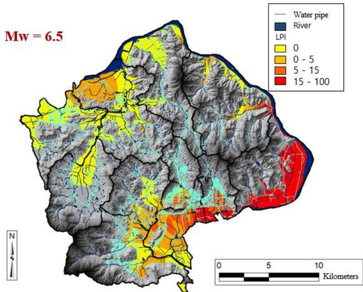
(b) Water pipelines superimposed on spatial distribution of LPI for  $M_w = 6.5$  earthquake
