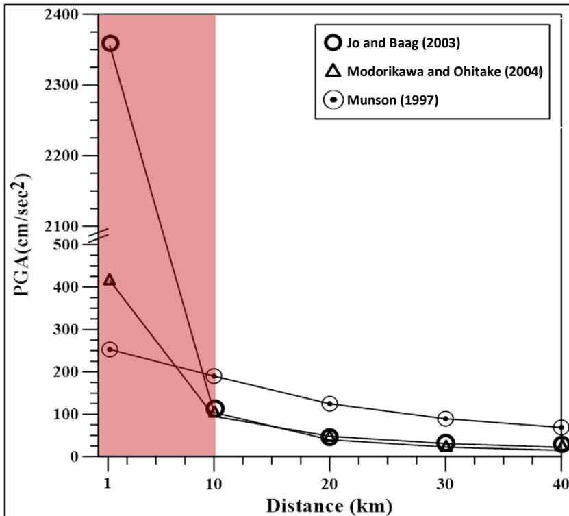
Figure 4. Peak ground acceleration (PGA) vs. distance from epicenter
