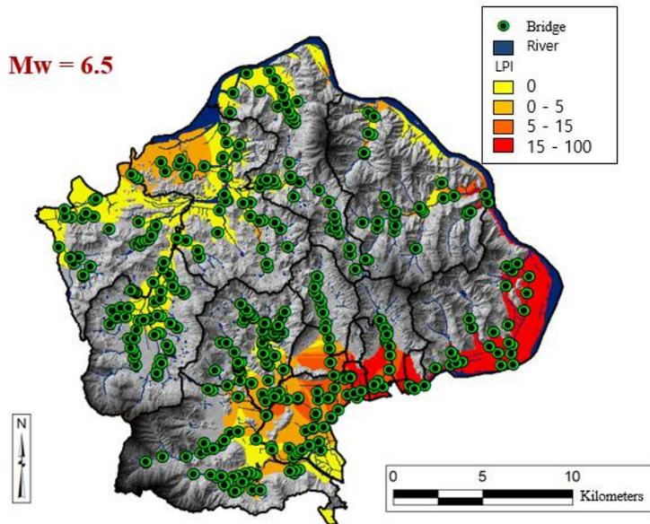
(b) Bridges superimposed on spatial distribution of LPI for  $M_w = 6.5$  earthquake
