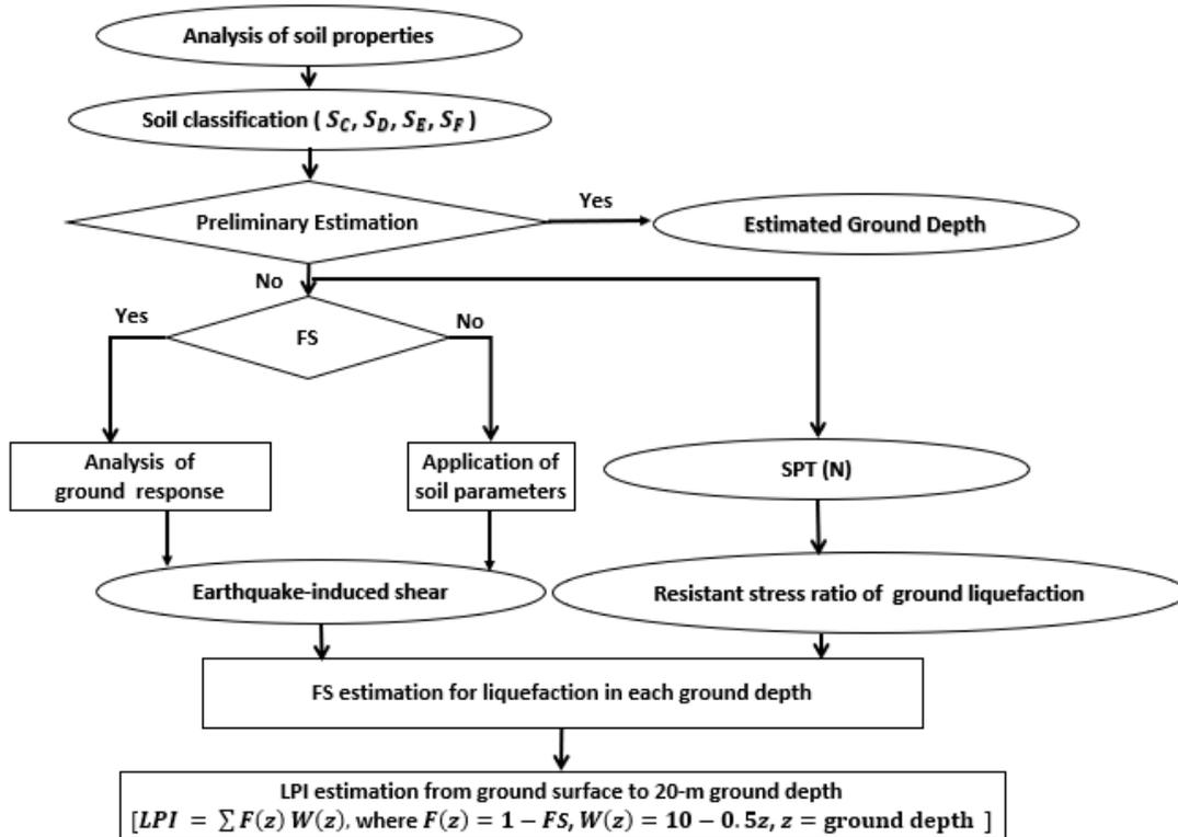
Figure 1. Flowchart for estimating liquefaction potential index (LPI) (Choe and Ku, 2009)
