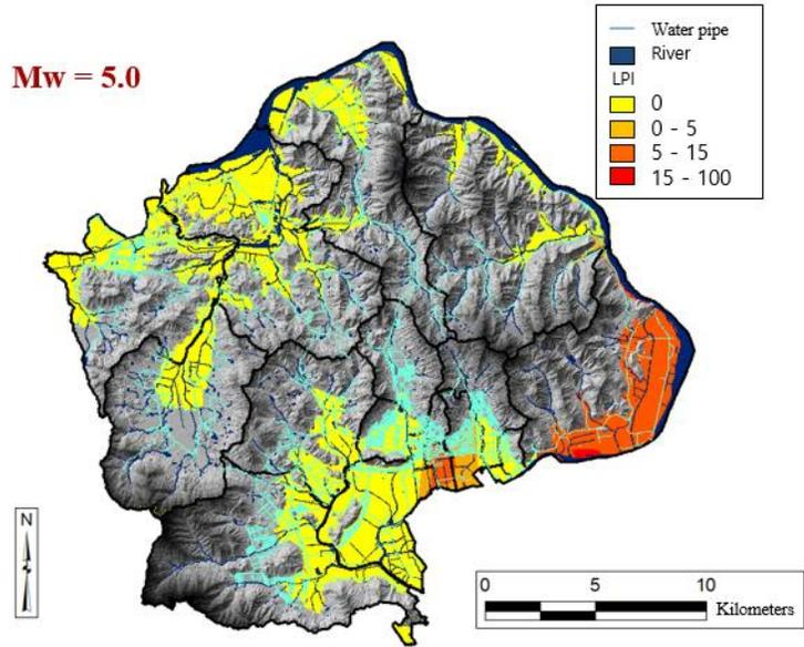
(a) Water pipelines superimposed on spatial distribution of LPI for  $M_w = 5.0$  earthquake
