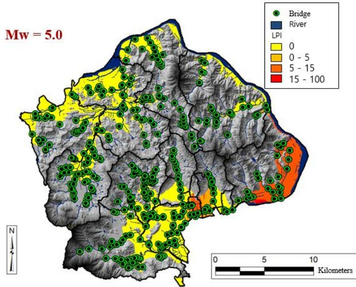
(a) Bridges superimposed on spatial distribution of LPI for  $M_w = 5.0$  earthquake
