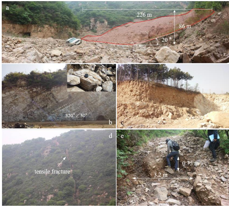
141 142 Fig.3 Field investigation photos. a Loose material; b Middle and Late Proterozoic dolomite; c colluvium deposit; d 143 Slope fracture; e Channel erosion phenomenon 144
