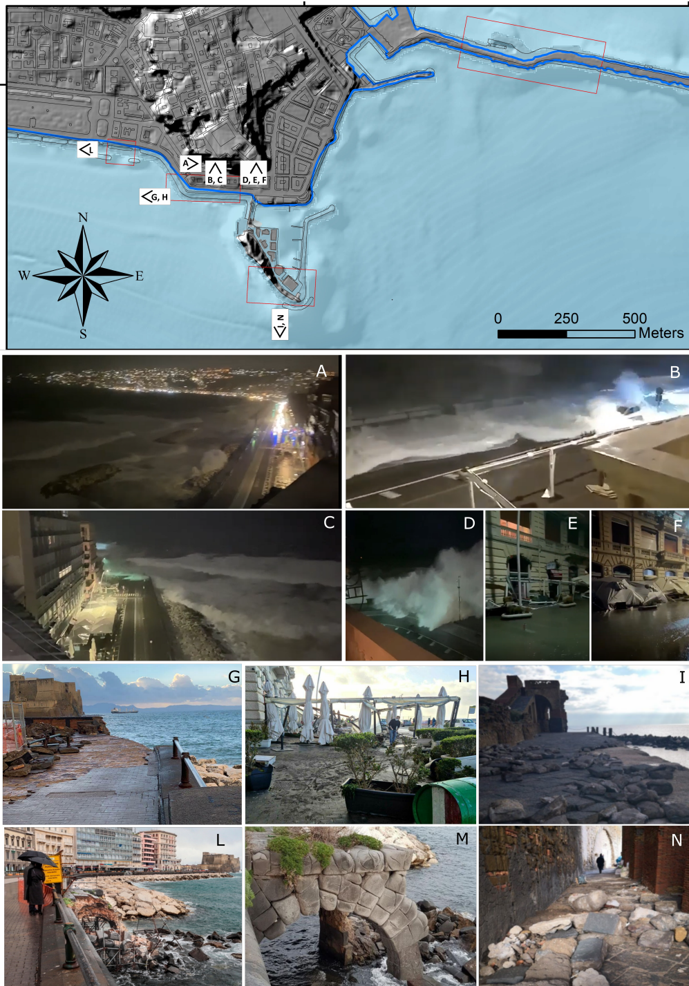
Figure 12. Photos of: A), B), C) and D) Storm surge in the coastal area with maximum setup values (Naples city center); E) and F) Damages on structures during the event; G) promenade destroyed with collapsed parapet; H) shattered shop windows; I) and N) Castel dell'Ovo after the event; L) and M) Bourbon pier after the event; H) Bourbon pier before the event.
