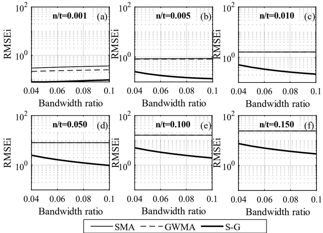
**Fig. 12** RMSEi for the harmonic scenarios on a semi-logarithmic scale
