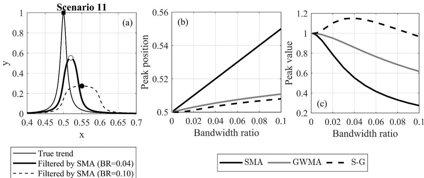
347 **Fig. 8** (a) An example of peak displacement by applying SMA, and variation of (b) peak position and (c)
