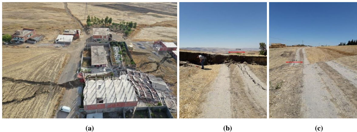
Figure 3. Ground cracks due to landslides in Kherba, Mila, ~2.5m offset towards the North, a. Drone aerial photo from (LNHC), b. & c.- Lateral displacements (Photos: courtesy M. Yacoub A., University of Setif, Algeria).
