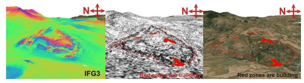
Figure 9. 3D view of Grarem Area, Images of IFG-3. Each fringe = wavelength/2 in LOS, and red zones represent existing building compounds (QGIS, ESRI basemap).
