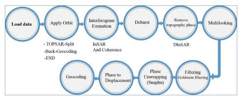
Figure 4. Workflow chart for the DInSAR processing using (SNAP) software.
