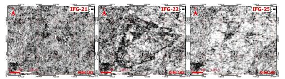
**Figure 8.** Coherence maps of Grarem AoI: the images represent pre-event (left), co-event (middle), and post-event (right) for orbits 66, 59, and 161. *Nota: the co-event maps for the three orbits show the decay of coherence that is triggered by the earthquake.*
