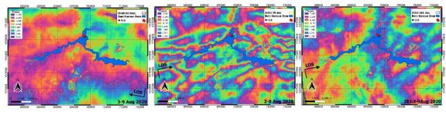
Figure 5. Wrapped Interferograms from Sentinel-1 for IFG-3+IFG-4, IFG-17 and IFG-22, The red star is the epicenter location (USGS).
