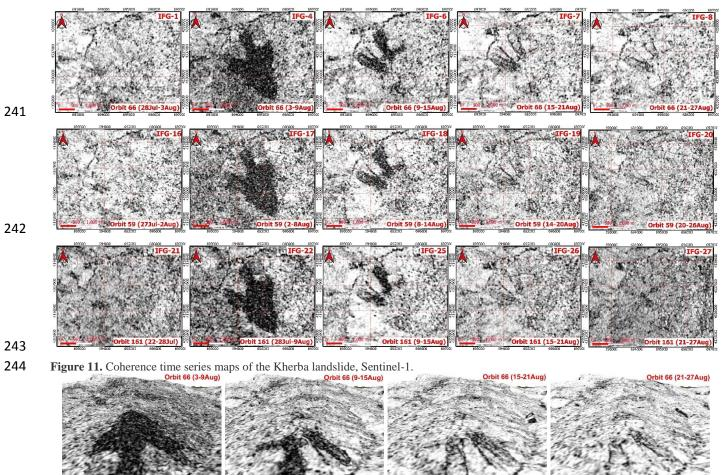
Figure 12. 3D view of Kherba landslide, Sentinel-1 Coherence images of Orbit 66 with a 6-day temporal baseline, the dark areas are the landslide and deformations zones.
