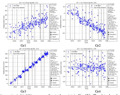
**Figure 19.** Displacement time series (orbit 161), corresponding to the points in Fig. 17.b, The plots show less dispersion of data points (linear) compared to short analysis, the long period analysis (5 years) is useful to eliminate other sources of noise.
