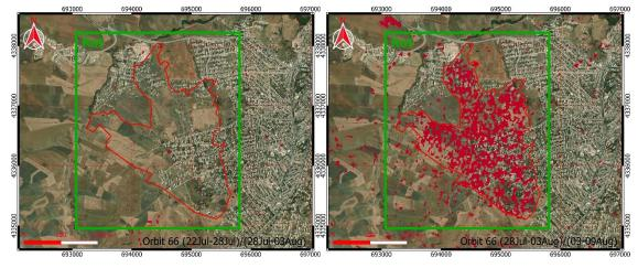
Figure 13. Pre-event coherences ratio (left), co-event coherences ratio (right), Sentinel-1 Orbit 66. The green box indicates the scope of the RoI, red spots represent significant changes of coherence in the landslide region (QGIS, ESRI World Imagery basemap).
