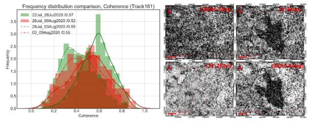
**Figure 15.** Effect of bad coherence: the cause is the acquisition of 3<sup>rd</sup> August start at (17:28:15, orbit 161) under bad weather conditions in the acquisition time according to precipitation site (WWO) (rainfall in that daytime), compared to the acquisition of the same day but not the same time (05:37:58 for orbit 66).
