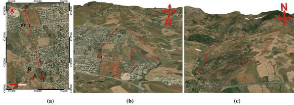
**Figure 2.** 3D view of AoIs, Kherba AoI and Grarem using QGIS with DEM SRTM 1sec and ESRI basemap, a & b are Kherba AoI, c is the Grarem case area, the red polygon is the boundary of change detected by InSAR.
