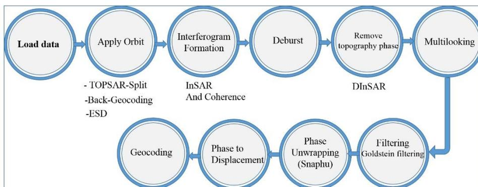
Figure 34. Workflow chart for the DInSAR processing using (SNAP) software.
