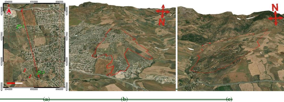
Figure 4. 3D view of AoIs, Kherba AoI and Grarem using QGIS with DEM SRTM 1sec and ESRI basemap, a & b are Kherba AoI, c is the Grarem case area, the red polygon is the boundary of change detected by InSAR.
