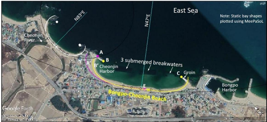
Figure 7: Aerial photograph of Bongpo-Cheonjin Beach in February 2021, showing harbors, river, shore protection structures and static bay shapes produced by software MeePaSoL on image courtesy of Google Earth.
