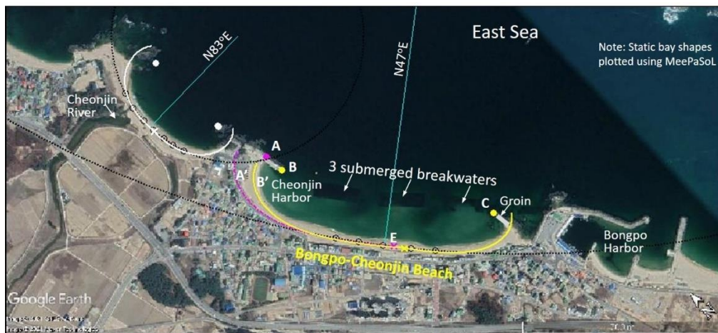
Figure 7: Aerial photograph of Bongpo-Cheonjin Beach in February 2021, showing harbors, river, shore protection structures and static bay shapes produced by software MeePaSoL © Google Earth.
