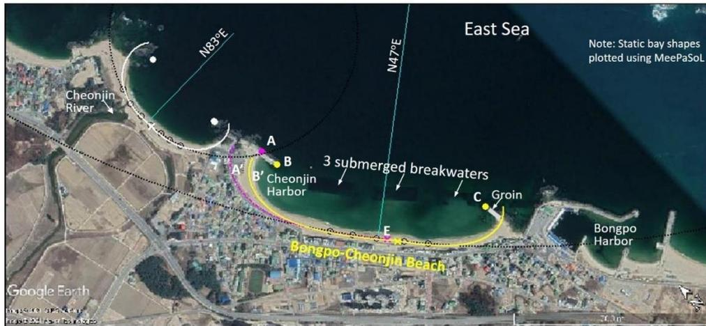
Figure 7: Aerial photograph of Bongpo-Cheonjin Beach in February 2021, showing harbors, river, shore protection structures and static bay shapes produced by software MeePaSoL on image courtesy of Google Earth.
