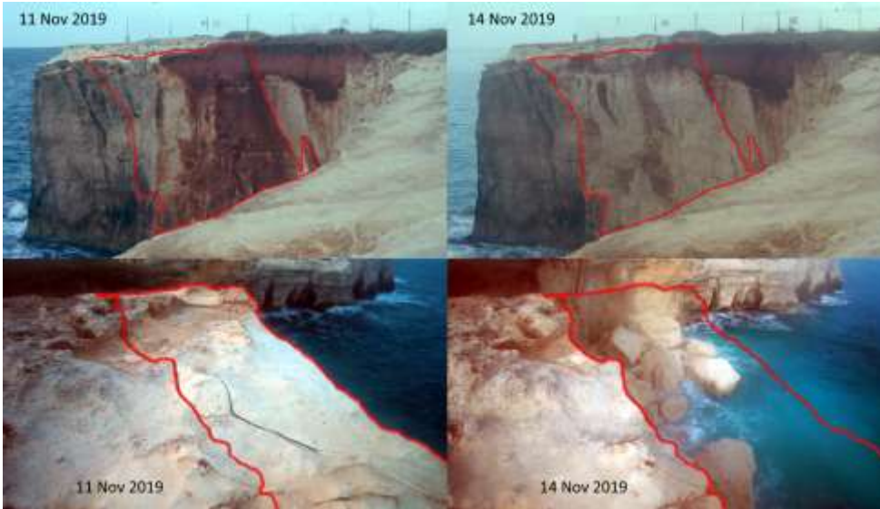
Figure 2: the first rockfall (marked with “A” on fig. 1) – Top left image shows the cliff as it was on 11 November 2019 and the top right image shows as it was 3 days later (both images are taken from the Raspberry Camera Module – see fig. 1 for the position). Bottom images shows the same event but from a different point of view (the secondary camera – see fig. 1 for the position): on the left, a picture taken before the collapse and on the right, a picture taken on 14 November 2019.
