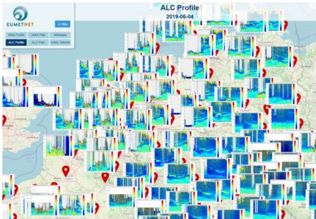
545 6 Figure 14: The E-PROFILE ALC network with quicklooks of attenuated backscatter observations from https://e-profile.eu . The quicklooks have time (0:00-24:00 UTC) on their x- and altitude above sea level (0-12 km) on their y-axis. The high values of attenuated backscatter correspond to clouds (orange and red) and aerosols (light blue, green and yellow). Low and mid-level clouds usually completely attenuate the signal above so that no observations above can be reported what is seen by the white areas in the quicklooks.
