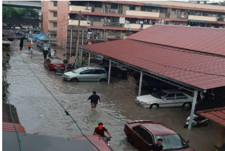
Figure 1: Pluvial Flood in Kampung Baru, 1 st October 2019. Due to poor drainage, water depth of 1 meter was reached after 2 hours of rain. (BERNAMA, 2019)
