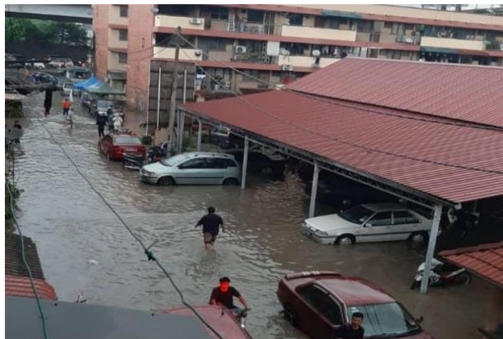
136 137 Figure 1: Pluvial Flood in Kampung Baru, 1 st October 2019. Due to poor drainage, water depth of 1 meter was 138 reached after 2 hours of rain. (BERNAMA, 2019) 139
