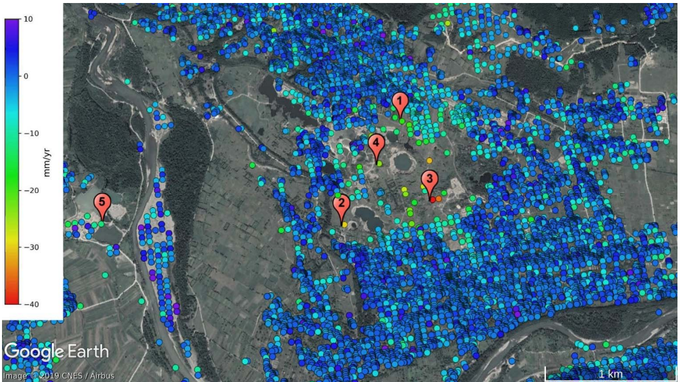
Figure 5: Linear rate of line-of-sight deformation from Sentinel-1 ascending pass for the investigated area (see explanation of numbers in the text). Contains modified Copernicus Sentinel data [2014-2019], background © Google.
