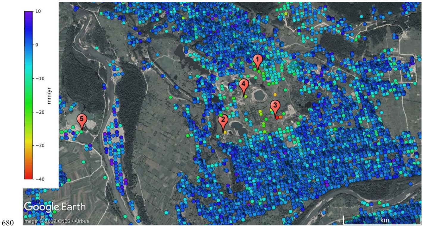
Figure 5: Linear rate of line-of-sight deformation from Sentinel-1 ascending pass for the investigated area (see explanation of numbers in the text). Contains modified Copernicus Sentinel data [2014-2019], background © Google.
