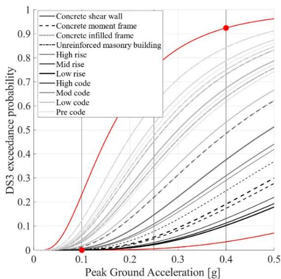
**Figure 3:HAZUS fragility curve database related to the Extensive Damage limit state for RC and URM buildings.**
