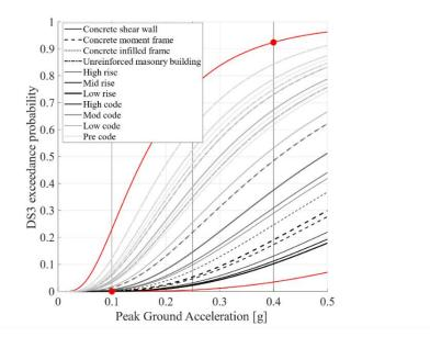
Figure 3:HAZUS fragility curve database related to the Extensive Damage limit state for RC and URM buildings.
