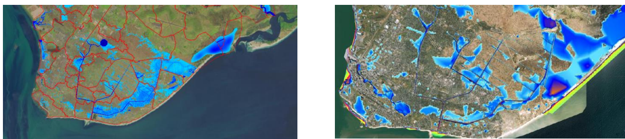
Figure 5 - flood extent resulting from a 10 year rainfall event for FLORES (left) and an ANUGA simulation, which was part of the Rio Chiveve feasibility study. Background image: Sentinel-2 (© ESA).
