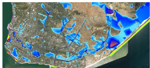
Figure 5 - flood extent resulting from a 10 year rainfall event for FLORES (left) and an ANUGA simulation, which was part of the Rio Chiveve feasibility study. Background image: Sentinel-2 (© ESA).
