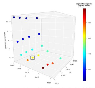
Figure 3 - Data analysis aimed at evaluating the best combination of bandwidth (hr) and threshold (th) values. The black rectangle identifies the selected combination.
