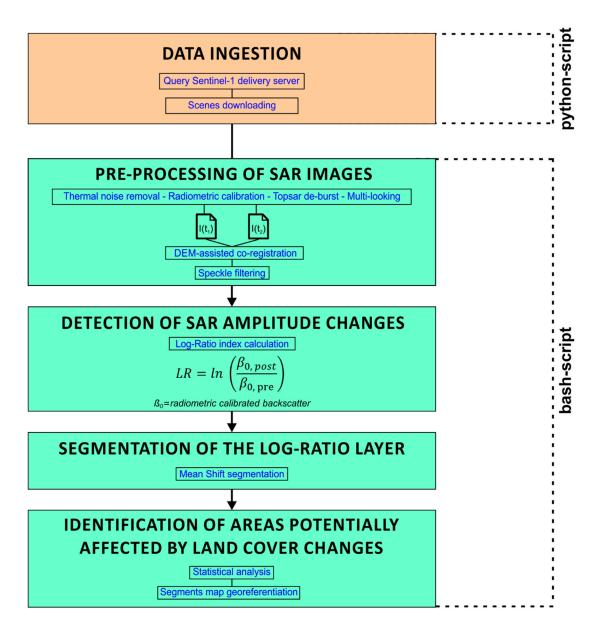
Figure 1: Flowchart of the automatic steps of the processing chain described in the text. The single steps are grouped in two main scripts (developed using Python and Bash scripting languages). I(t<sub>1</sub>) and I(t<sub>2</sub>) represent two consecutive SAR images (or set of images).
