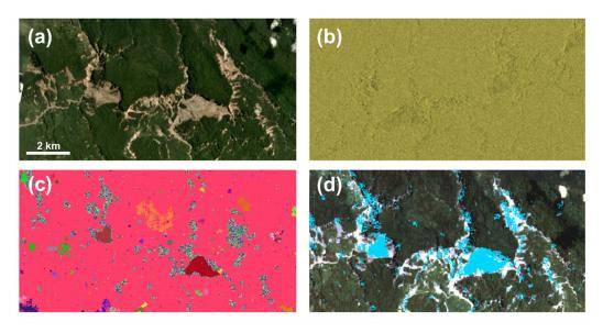
Figure 4 - a) Optical image of a small sample area affected by landslides within the AoI; b) the corresponding Log-Ratio layer; c) the output of the segmentation algorithm (obtained using the optimized hr and th values); d) the extracted landslide-related segments (in blue).
