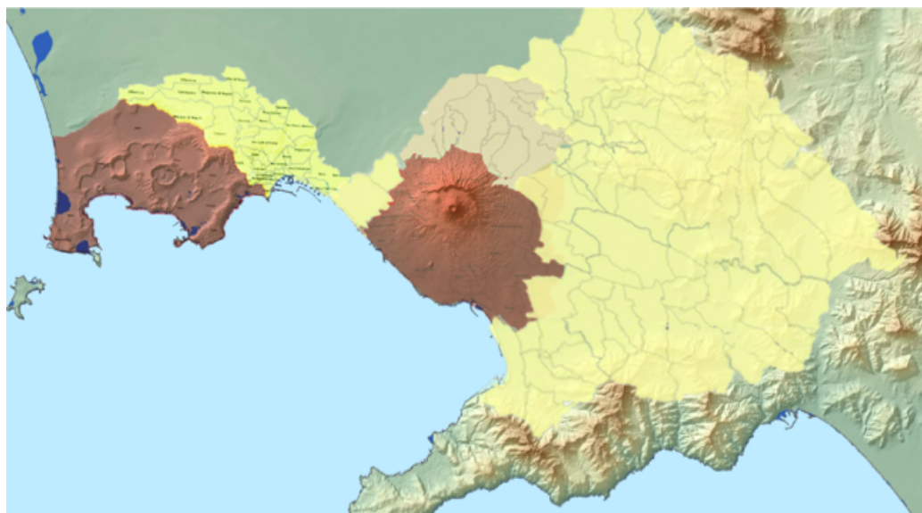
Figure 5: Red and Yellow zones for Campi Flegrei and Vesuvius. Red zones are the areas with maximum pyroclastic flow hazard, which have to be completely evacuated within 72 hours from the declaration of 'Red alert'. Yellow zones are the areas with maximum hazard for accumulation of pyroclastic falls on flat roofs (visit http://www.protezionecivile.gov.it/risk-activities/volcanic-risk/italian-volcanoes )
