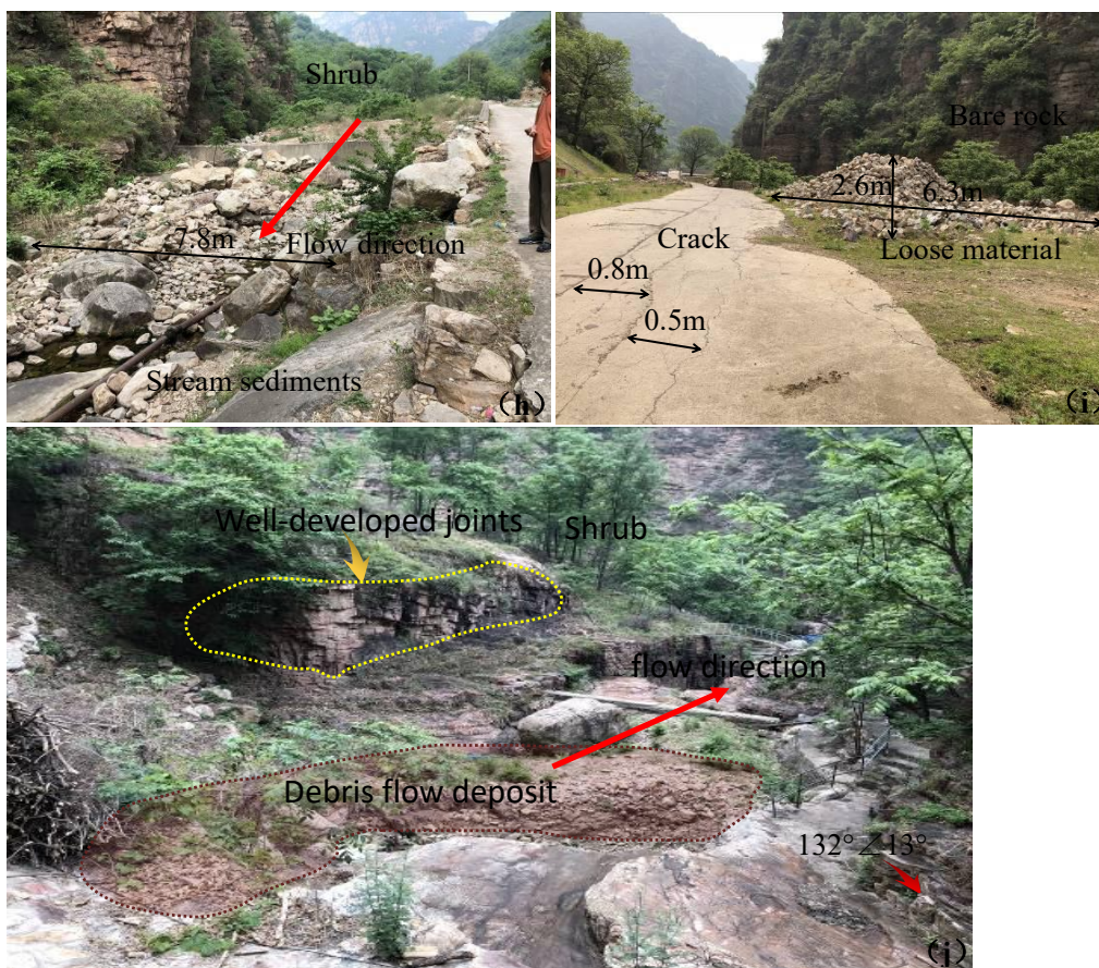
130 Fig.5 Lishu scenic spot. h stream sediments, i road cracks, g debris flow deposit.
