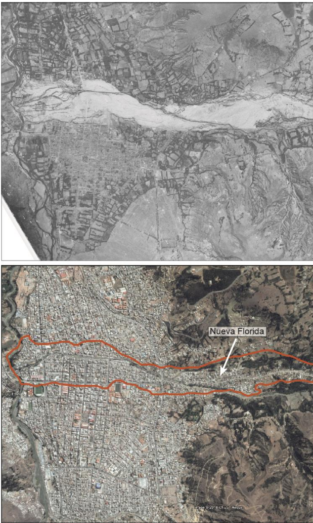
Figure 6: Aerial photograph from 1948 showing the traces of the 1941 GLOF (upper panel), and 2016 satellite image of the same area (lower panel). The outlines in orange indicate the extent of the area affected by the 1941 GLOF. The
