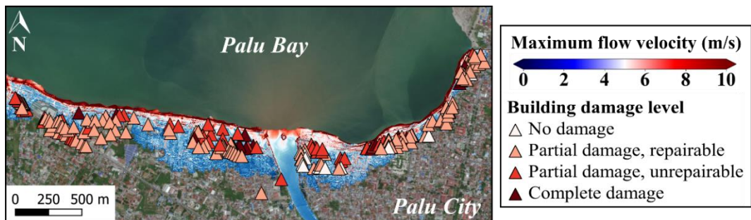
660 Figure C3. Sulawesi-Palu final tsunami inundation model with the maximum simulated flow velocity overlaying on the damaged building data (background ESRI).
