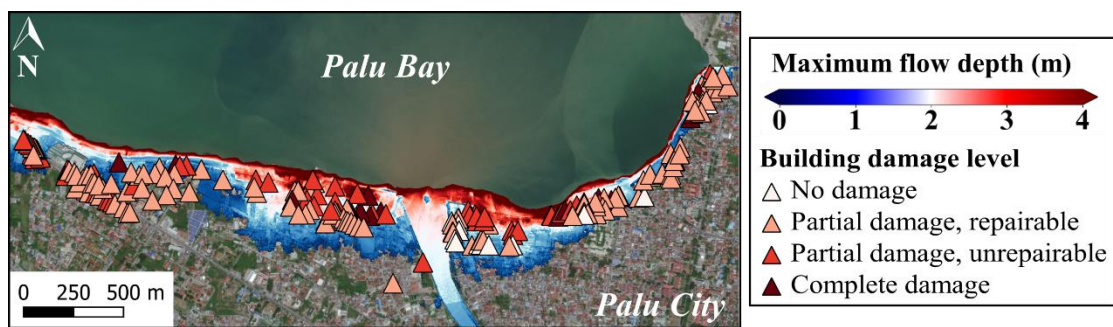
Figure 8. Sulawesi-Palu final tsunami inundation model with the maximum simulated flow depth overlaying on the damaged building data (background ESRI).
