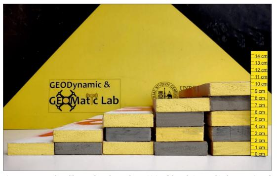
Figure 11: Rectangular calibres made to observe the sensitivity of the technique used in the comparison of point clouds.
