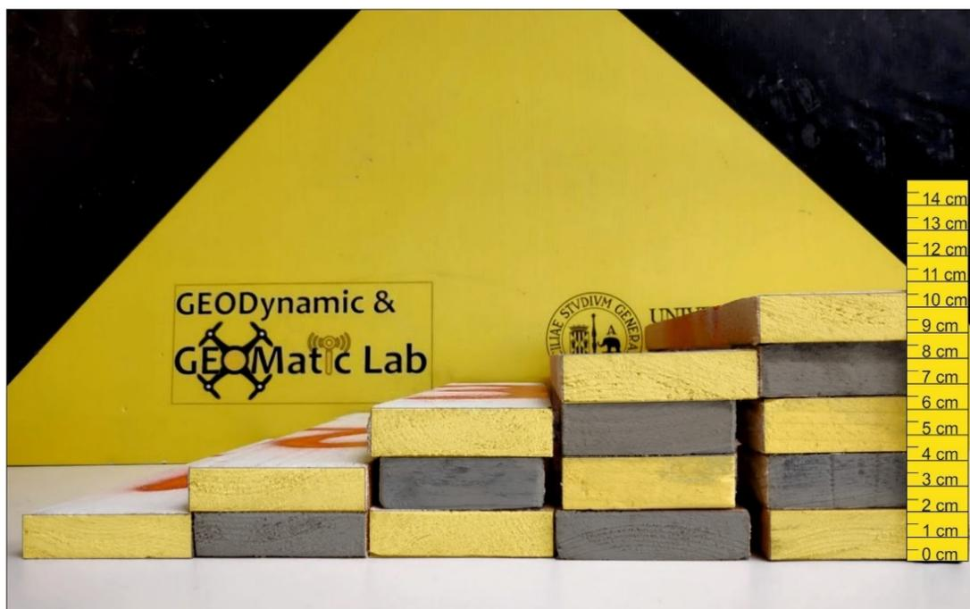
Figure 11: Rectangular calibers made to observe the sensitivity of the technique used in the comparison of point clouds.
