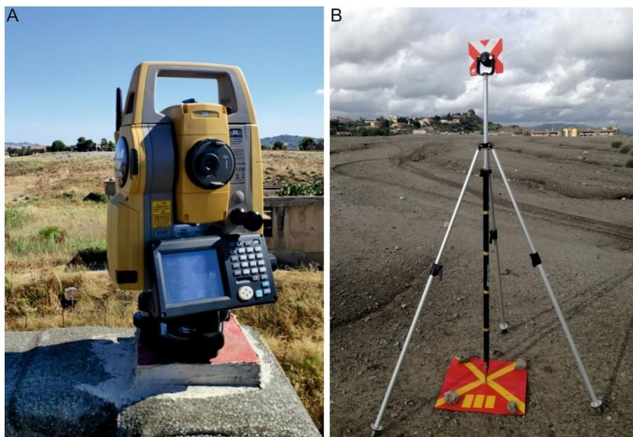
150 **Figure 5: A) TST DS 103 placed on the fixed metal base in coincidence with point CTN0. B) Surveying ranging rod on the mud volcano during the survey phase.**
