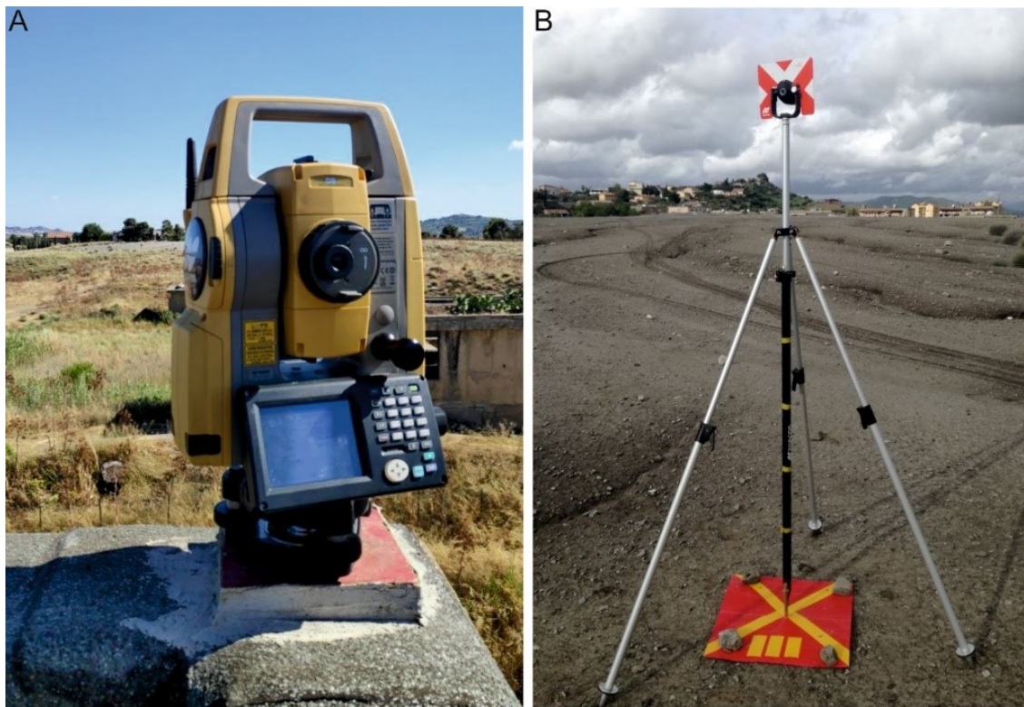
165 Figure 5: A) TST DS 103 placed on the fixed metal base in coincidence with point CTN0. B) Surveying ranging rod on the mud 170 volcano during the survey phase.
