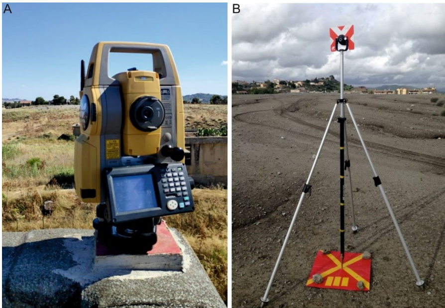
165 Figure 5: A) TST DS 103 placed on the fixed metal base in coincidence with point CTN0. B) Surveying ranging rod on the mud volcano during the survey phase.
