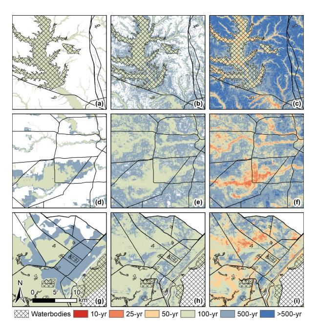
**Figure 5.** Side-by-side visual comparison for three areas affected by differing flood types. (a-c) Conroe area (d-f) Meyerland and (g-i) Port Arthur. Maps compare (left) current effective 100-year and 500-year flood plains (c. 2016) (center) areas within the 100-year and 500-year annual flood zones based on the Random Forest flood model;(right) continuous flood hazard map. Road layers originated from the U.S. Census Bureau and Floodplains originated from Federal Emergency Management Agency.
