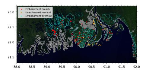
**Figure 8.** Digitized location of inundation resulting from embankment breaching (red), flooding of low-lying unembanked area (orange), and embankment overflow (cyan) overlaid on a false-colour image composite derived from B12, B11, and B4 channels of Sentinel-2 during April 2020. The grey patches are the inundated regions predicted by the model, as shown in the hindcast experiment. The polders are shown with cyan outlines.
