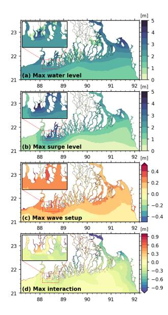
**Figure 5.** Hindcast of (a) maximum water level, (b) maximum surge (c) wave setup/setdown (d) maximum non-linear interaction between tide and surge. For (a), for the areas above mean sea level, the water level is converted to water level above the topography for consistency. The inset maps show a close-up (75 km  $\times$  45 km) of the landfall region.
