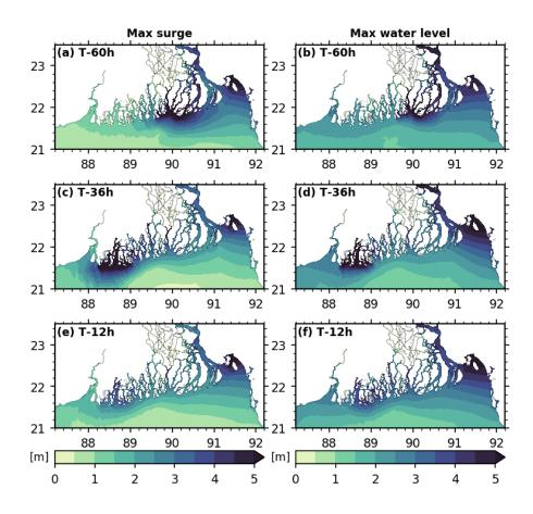
**Figure 7.** Maximum surge (a, c, e) and elevation (b, d, f) evolution for forecast initiated at (a-b) T-60 hours (2020-05-18 0000Z), (c-d) T-36 hours (2020-05-19 0000Z), (e-f) T-12 (2020-05-20 0000Z) hours before landfall.
