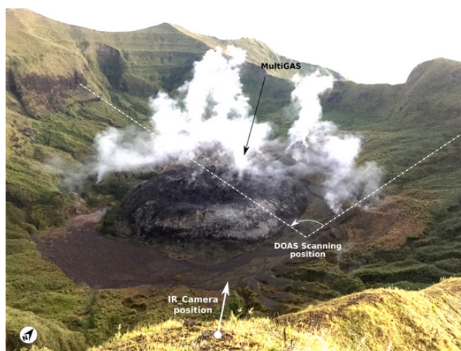
Figure 2. Awa lava dome in the crater. Degassing occurs from the lower crater wall and the northern part of the crater is the main degassing zone. The positions of DOAS scanning, MultiGAS (MG) and Infrared Camera are highlighted. The arrow of the IR_cam denotes the direction of the thermal camera.
