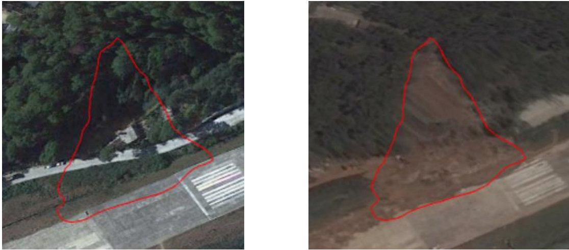
Figure 1: Pre Mangkhut (a and c) and post (b and d) images from Baguio airport runway landslide. Images a) and b) are an orthophoto, c) and d) are Google Earth images (note that North is at the bottom right of the picture).
