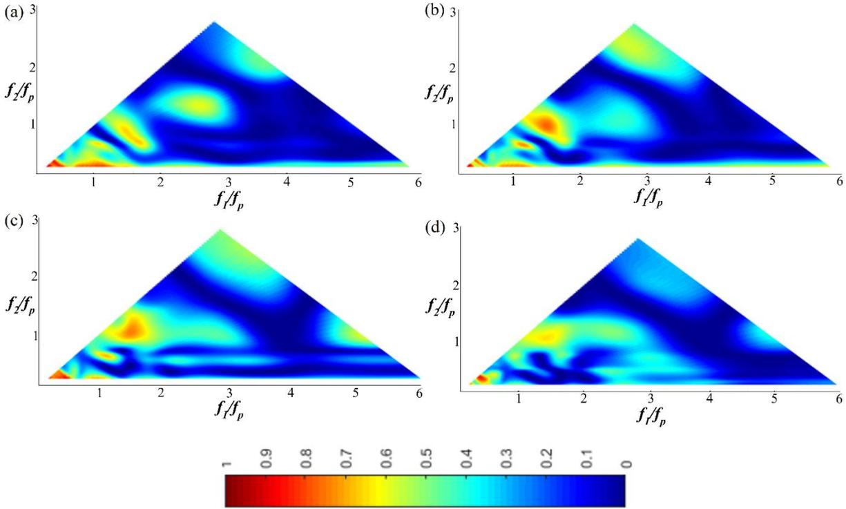
235 **Figure 6 : The wavelet-based bicoherence spatial evolution on the sloping bottom for a Pierson-Moskowitz wave train (Test 3). (a):**
