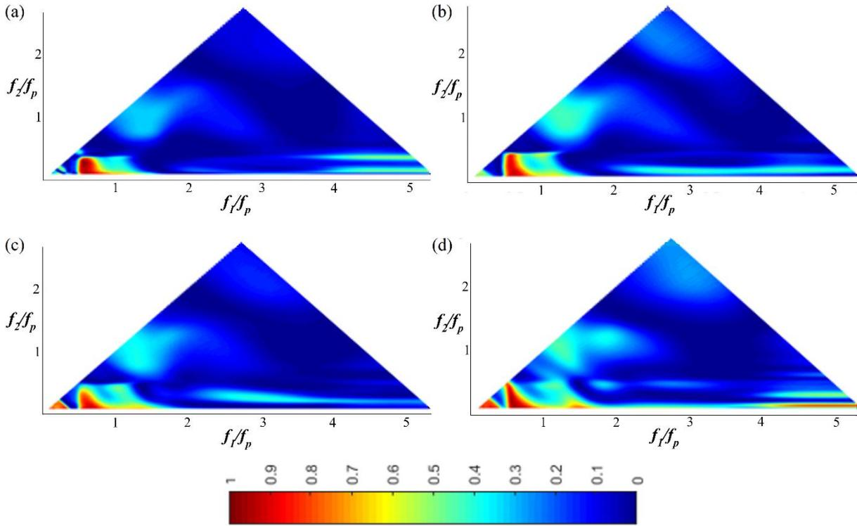
290 **Figure 9: The wavelet-based bicoherence spatial evolution on the flat bottom for JONSWAP ( $\gamma = 7$ ) wave train (Test 7). (a):  $x = 4$  m; (b):  $x = 6.4$  m; (c):  $x = 8$  m; (d):  $x = 9.6$  m.**
