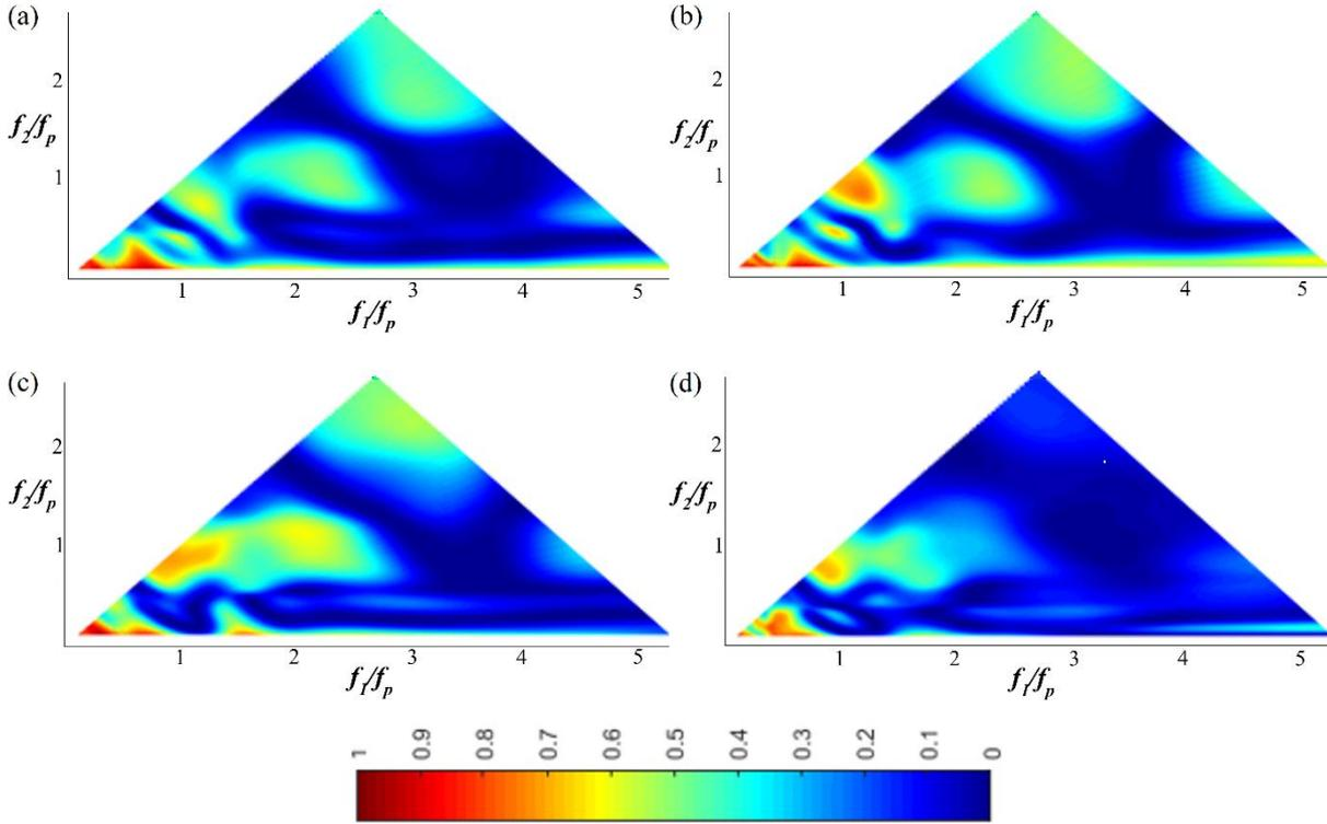
**Figure 8: The wavelet-based bicoherence spatial evolution on the sloping bottom for JONSWAP ( $\gamma = 3.3$ ) wave train (Test 5). (a):  $x = 10.20$  m; (b):  $x = 11.20$  m; (c):  $x = 12.40$  m; (d):  $x = 13.60$  m.**
