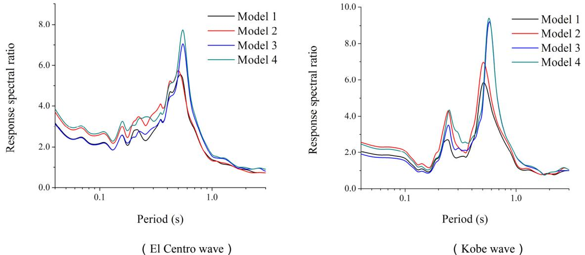
**Figure 5.** Response spectral ratio between the surface and the base input of SV wave form
