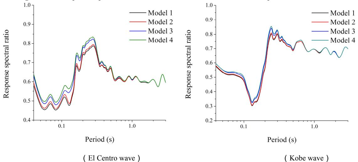
**Figure 6.** Response spectral ratio between the surface and the base input of P wave form
