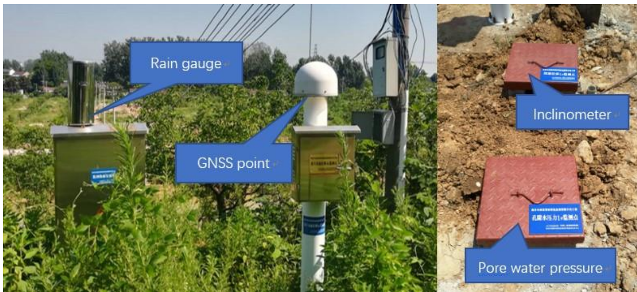
Figure 3 Monitoring instruments on the landslide
