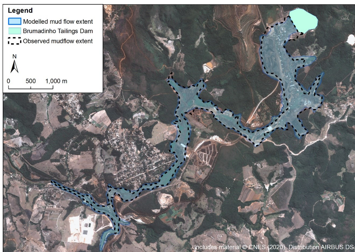
Figure 6: Comparison of the maximum modelled mud extent and the observed maximum mud extent downstream of the Brumadinho tailings dams
