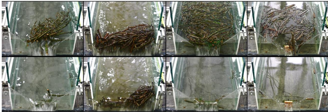
Figure 11: Characterizing release conditions: a) dimensionless overtopping depth h^* VS buoyancy to drag force ratio \Pi/F_D with dot size and opacity proportional to the amount of LW released. Inset: same figure with non-logarithmic x-axis highlighting the sharp increase in h^* for significant releases; and (b-e) pictures of selected releases before (top picture) and after (bottom picture) releases. Releases occur for lower h^* in the \Pi/F_D \gg 1 domain, i.e., if buoyancy prevails and floating carpets forms with loosely packed logs (see d & e); while releases
