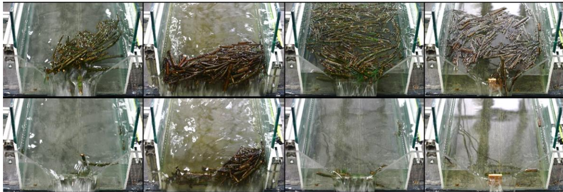
Figure 11: Characterizing release conditions: a) dimensionless overtopping depth h^* VS buoyancy to drag force ratio \Pi/F_D with dot size and opacity proportional to the amount of LW released. Inset: same figure with non-logarithmic x-axis highlighting the sharp increase in h^* for significant releases; and (b-e) pictures of selected releases before (top picture) and after (bottom picture) releases. Releases occur for lower h^* in the \Pi/F_D \gg 1 domain, i.e., if buoyancy prevails and floating carpets forms with loosely packed logs (see d & e); while releases
