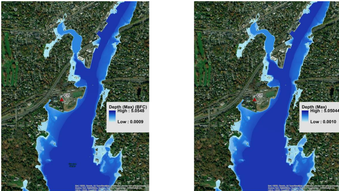
Figure R2: Maximum flood depth during the actual Irene event: left: streamflow with DCT, right: Streamflow without DCT, as presented in the submitted manuscript.
