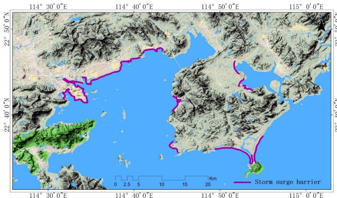
170 **Figure 2.** The map of the study area including the Storm Surge Barriers such as dikes and levees along the coastline of Huizhou, which are indicated by the violet lines. The map was made with ArcGIS 10.5 software based on the terrain base map layer, which was obtained from Google Maps (Map data ©2019 Google).
