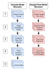
Figure 1: Two types of model structures as introduced by Trigg et al. (2016), with the cascade model structure in blue and the gauged flow model structure in red.
