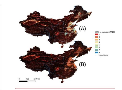
Figure 2: Aggregated flood hazard maps for both flood types, where the numbers and corresponding colors indicate the number of models in agreement on the inundation of a grid cell. 2a: Aggregated undefended fluvial flood hazard maps of 7 GFMs for RP100. 2b: Aggregated undefended combined (fluvial and pluvial) flood hazard maps of 3 GFMs for RP100.
