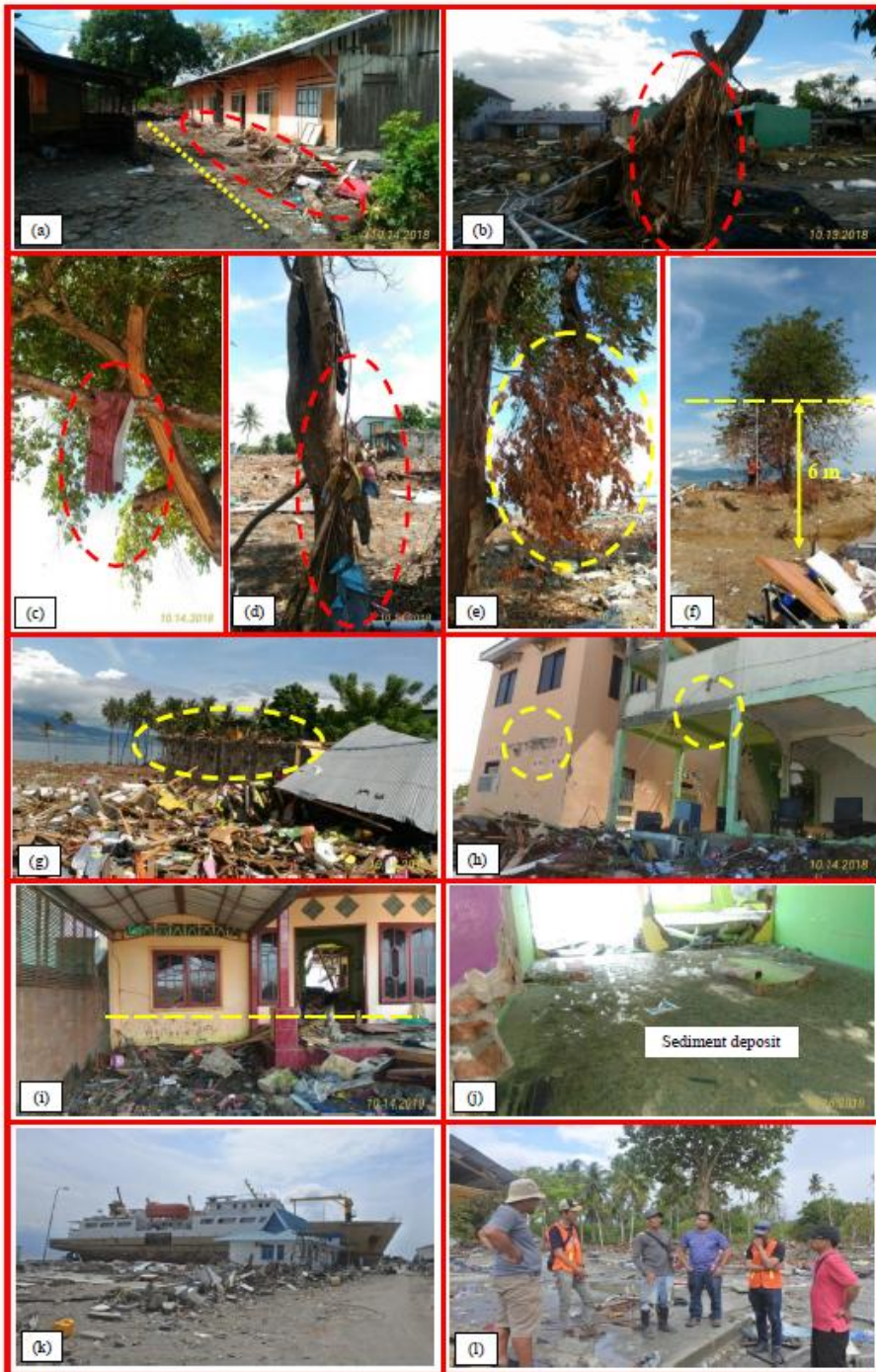
Figure 2: Evidence of tsunami runup and inundation. (a) Debris left behind in the residential area of Tondo, (b) debris caught in a tree in Mamboro, (c) and (d) debris stuck in a tree in Tondo, (e) leaves turned brown due to being submerged in salt water, (f) a tree had green leaves at the top and brown at the lower part, indicating the tsunami inundation height (flow depth) limit in Layana, (g) debris lodged on top of a building, (h) broken house element showing tsunami water level, (i) watermark on a house wall in Lero village, (j) sand deposit on building floor in Donggala City, (k) a 45-m-long ship moved to land in Wani harbour, (l) interview with an survivor in Mamboro.
