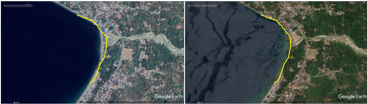
Figure 13: Quick land subsidence in Lero Village. Satellite images taken on (a) 7 April, 2016, and (b) 2 October, 2018, from Google Earth, showing conditions after the earthquake and tsunami. The area of land that dropped is 22,971 m 2 or almost 2.3 hectares.
