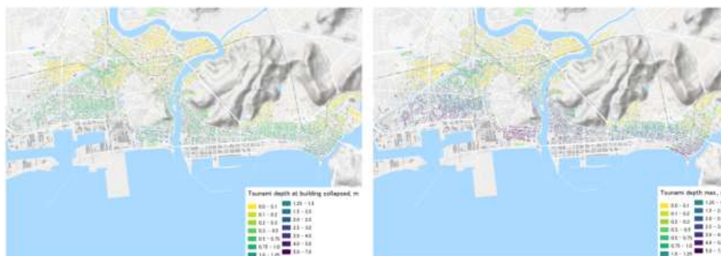
Fig. 10 Distribution of the critical flow depth (left) and the maximum flow depth (right)
