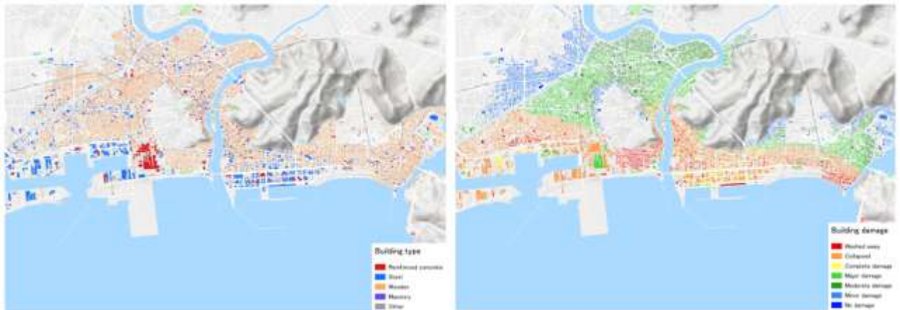
186 187 Fig.2 (Left) Distributions of building types and (Right) building damage levels.
