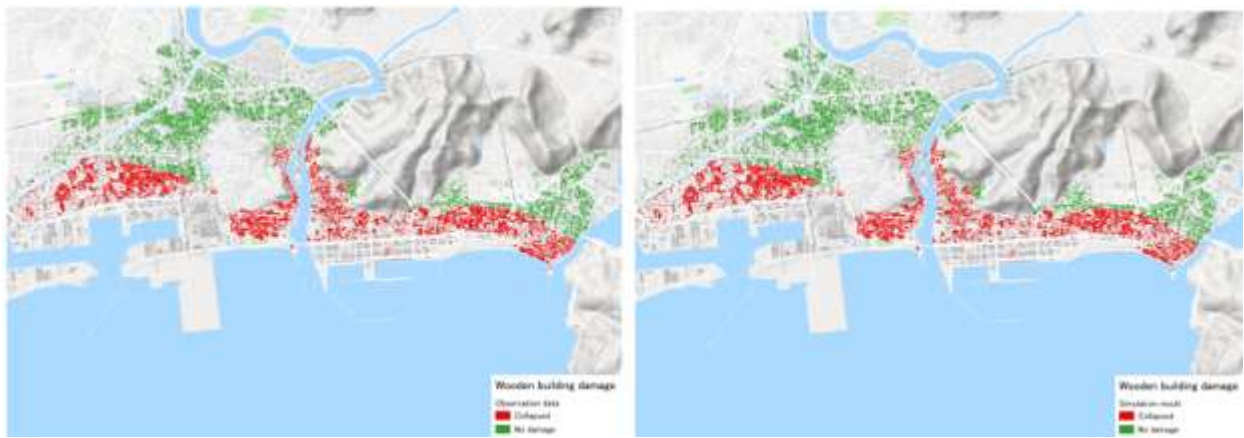
362 Fig. 9 Distributions of collapsed and non-collapsed buildings from field observation (left) and the 363 proposed method (right)
