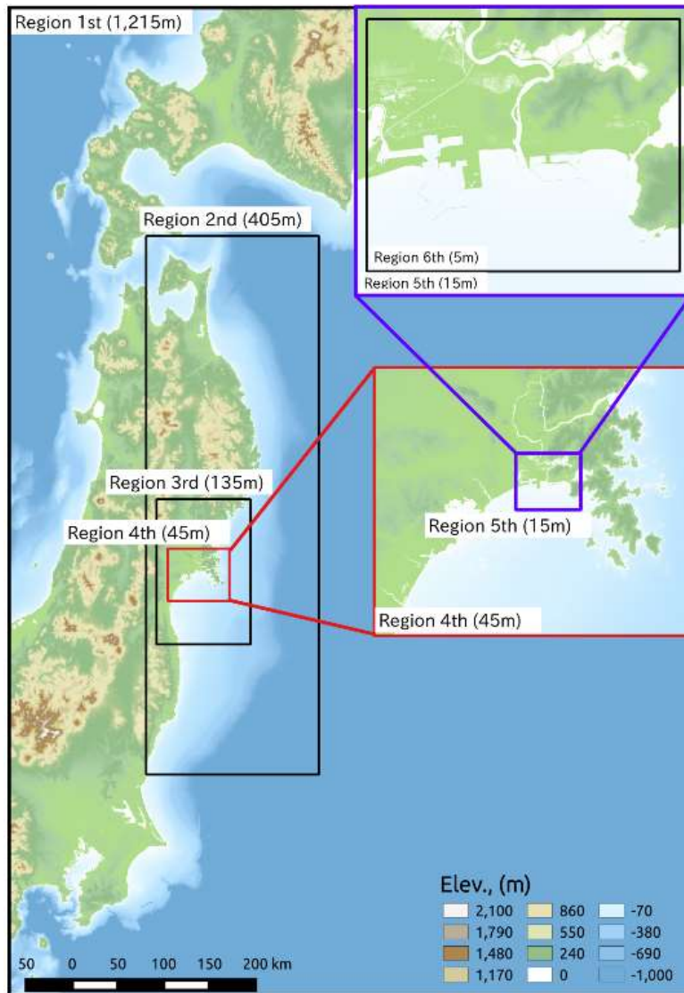
Fig.4 Computational regions in this study. Projection of bathymetry and topography data is the Japanese Geodetic Datum 2000 and the Tokyo Peil (T.P.) datum.
