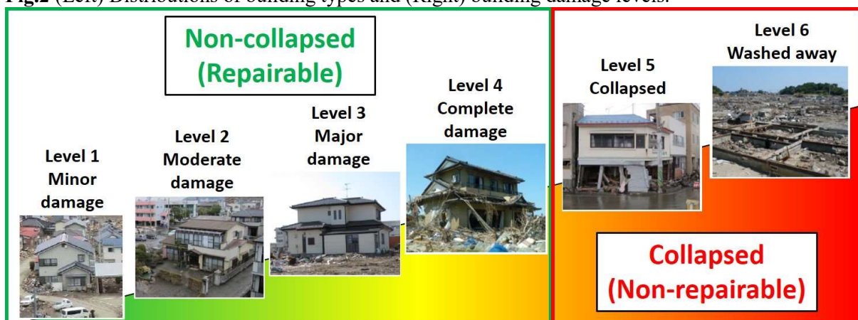
188 189 Fig. 3 Building damage levels and collapsed condition considered in this study (courtesy of MLIT, 190 2012).
